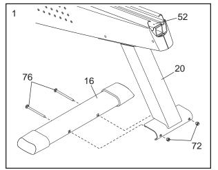
Orient the Front Stabilizer (15) as shown. While another person lifts the front of the Frame (1), attach the Front Stabilizer to the Frame with two M10 x 112mm Carriage Bolts (76) and two M10 Nylon Locknuts (72).
